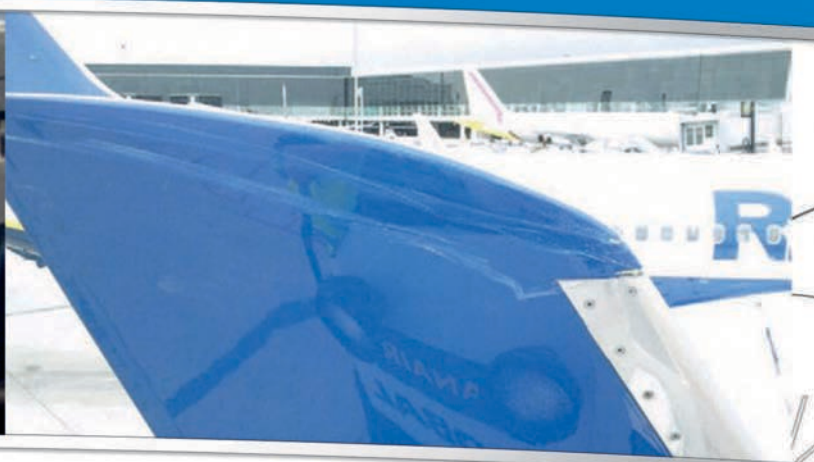
→ The damage of the right hand winglet of EI-EKB Photo: CIAIAC
