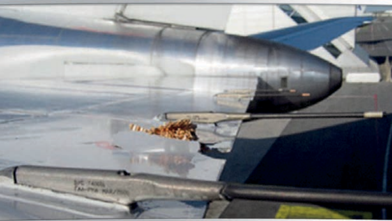
→ The damage of the left hand elevator/stabilizer of N366AA, photo taken at stand 41 at JFK Photo: CIAIAC
